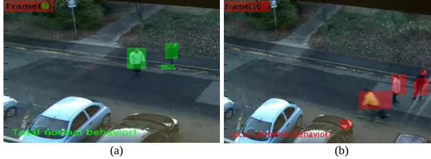
Fig. 12. Detection of behavior by fuzzy logic in dataset BMVA, (a) normal behavior, (b) abnormal behavior.
