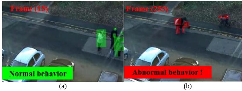
Fig. 10. Example 1 of event detected by fuzzy logic in dangerous situations (a- normal behavior, and b- abnormal behavior).
