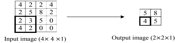
Fig. 3. The max-pooling operation.
