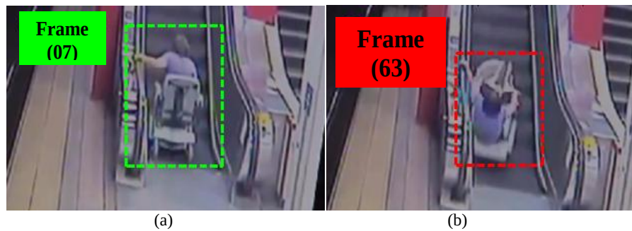
Fig.11. Example 2 of event detected by fuzzy logic in situation in an escalator (a- normal behavior, and b- abnormal behavior).
